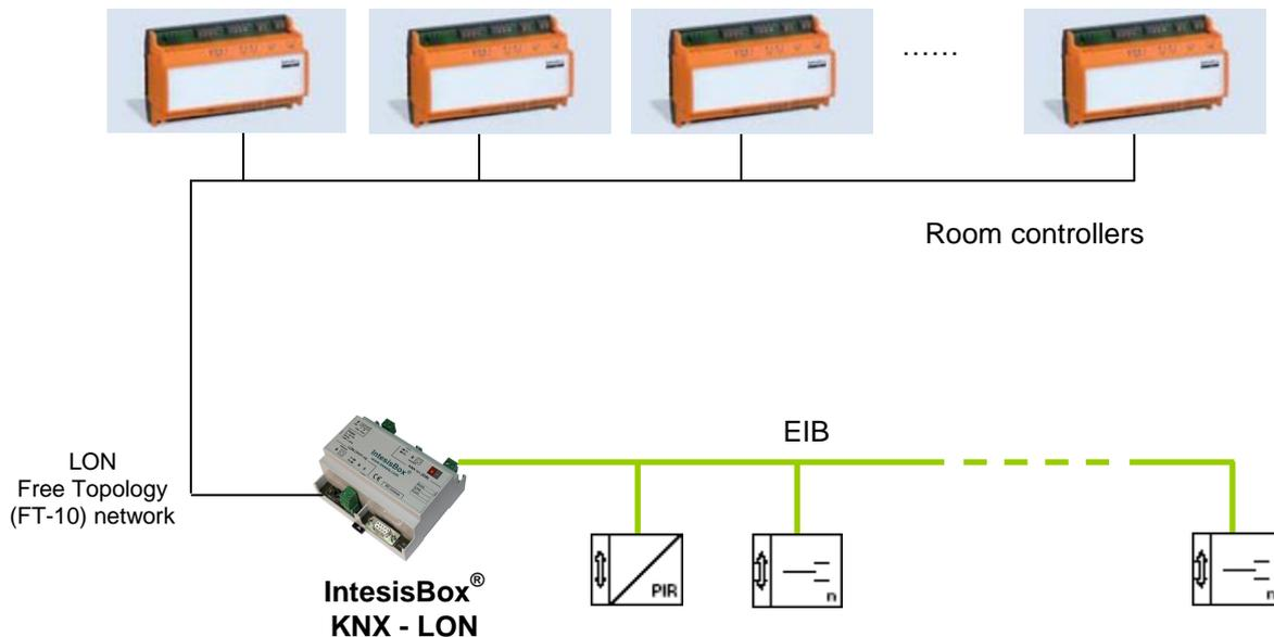
LON network variable interface for each particular LON room controller should be mapped into IntesisBox configuration. *LinkBoxEIB* software eases this task by providing a list of standard network variable types (SNVTs), with their respective fields, which can be assigned to each point.
