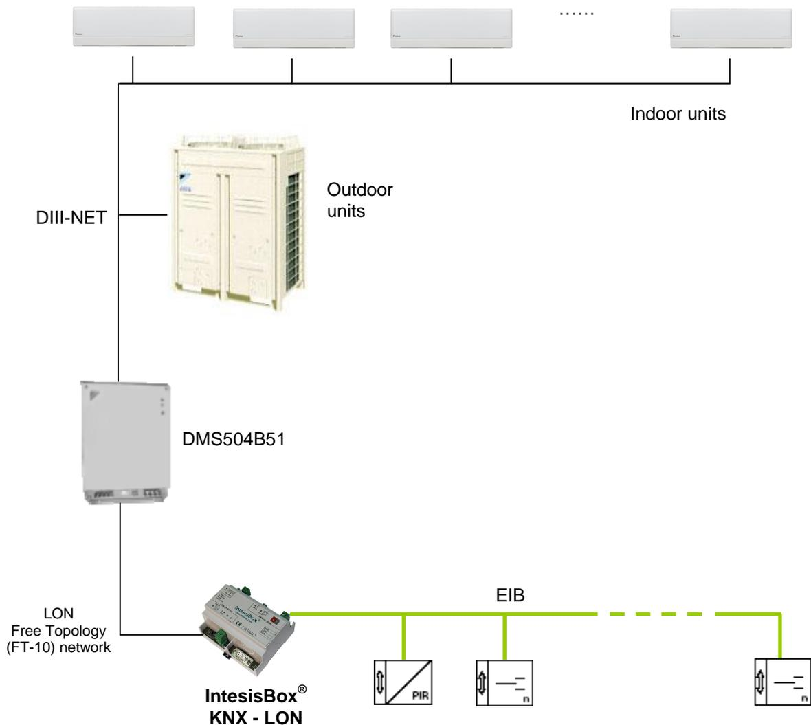
In the technical documentation of IntesisBox, supplied with the device, extended details on how to configure IntesisBox for this application are provided.
